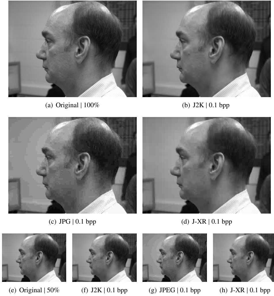
Figure 12: Maximum compression with JPEG2000, JPEG and JPEG-XR S_1 (b)-(d) and S_2 (f)-(h) for full profile images (a) and (e) on sample image ID_02463d677 of the UND dataset.
